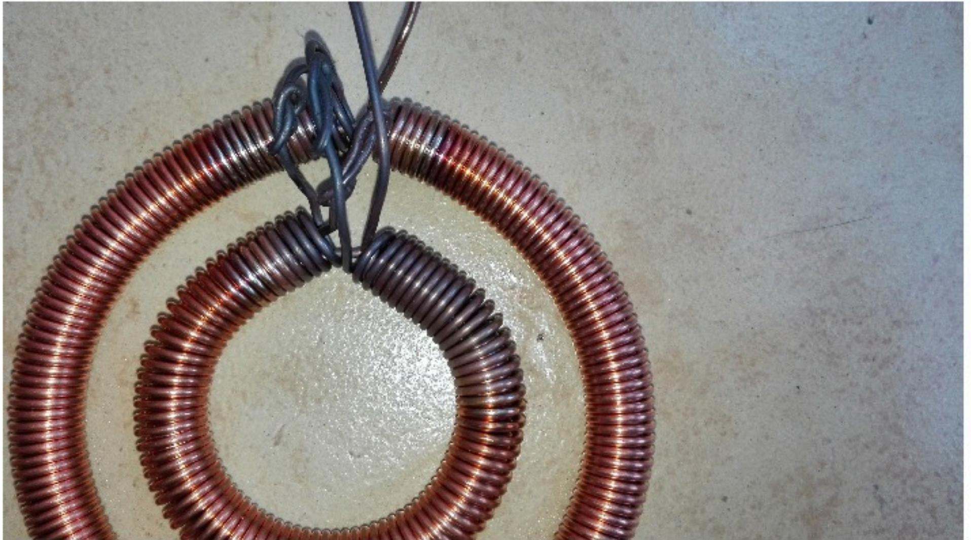
Move the flame towards the center loop and start moving clockwise slowly maintaining the desired temperature while moving along the coil.
