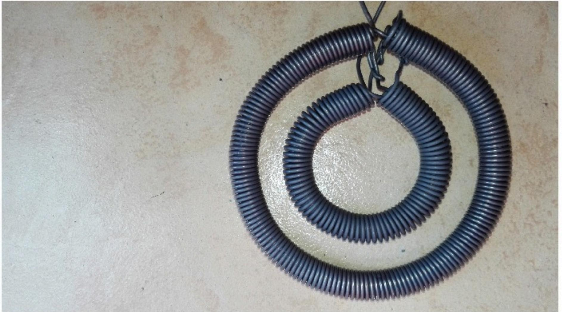
After cooled down by itself, one can make corrections on form then repeat the heating process one last time and it will be ready for use after cooling itself. Just leave it on the same tile while cooling.
