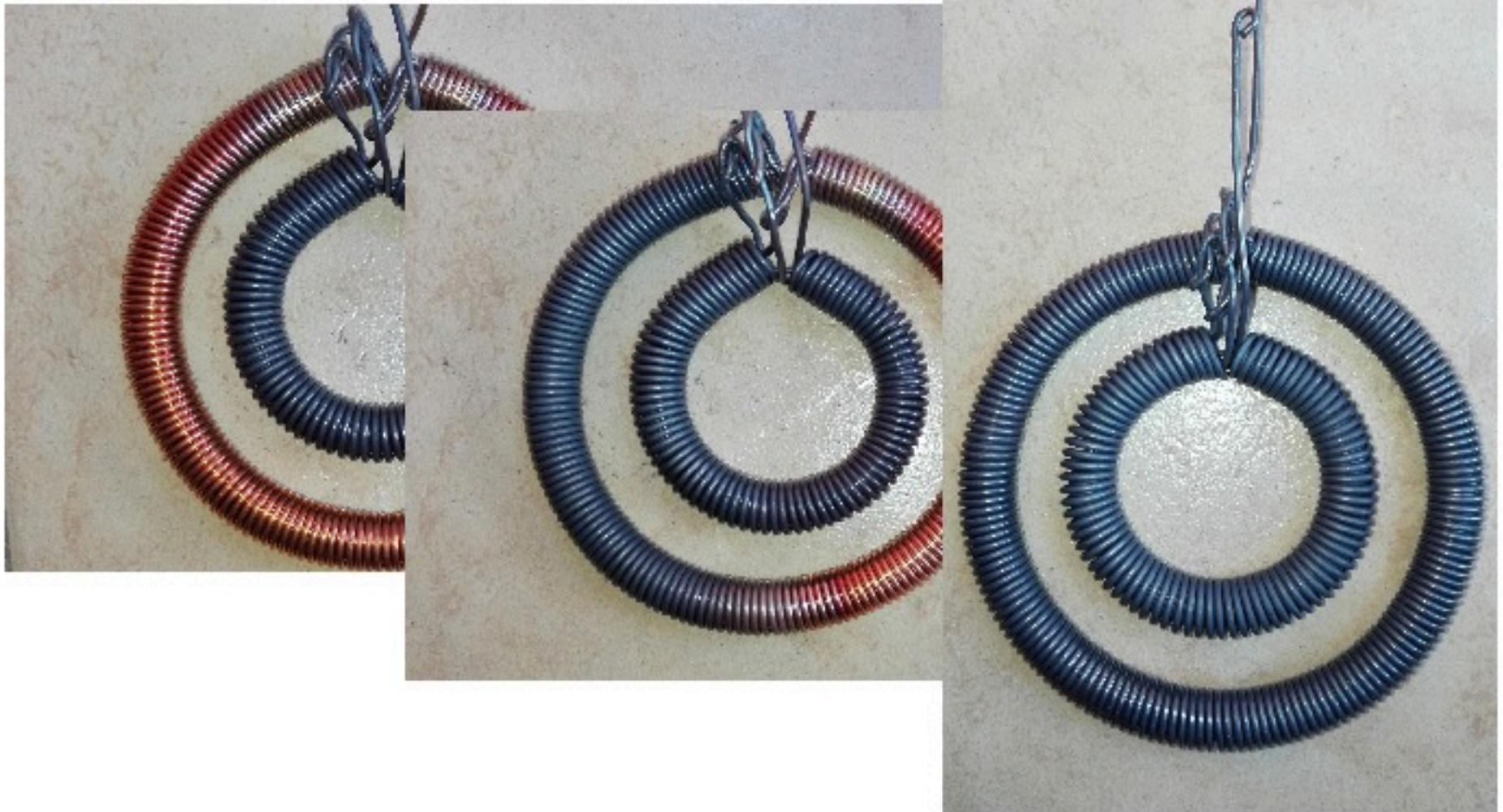
Start on the wire junction, temperature should be only be right before copper turns red hot.
