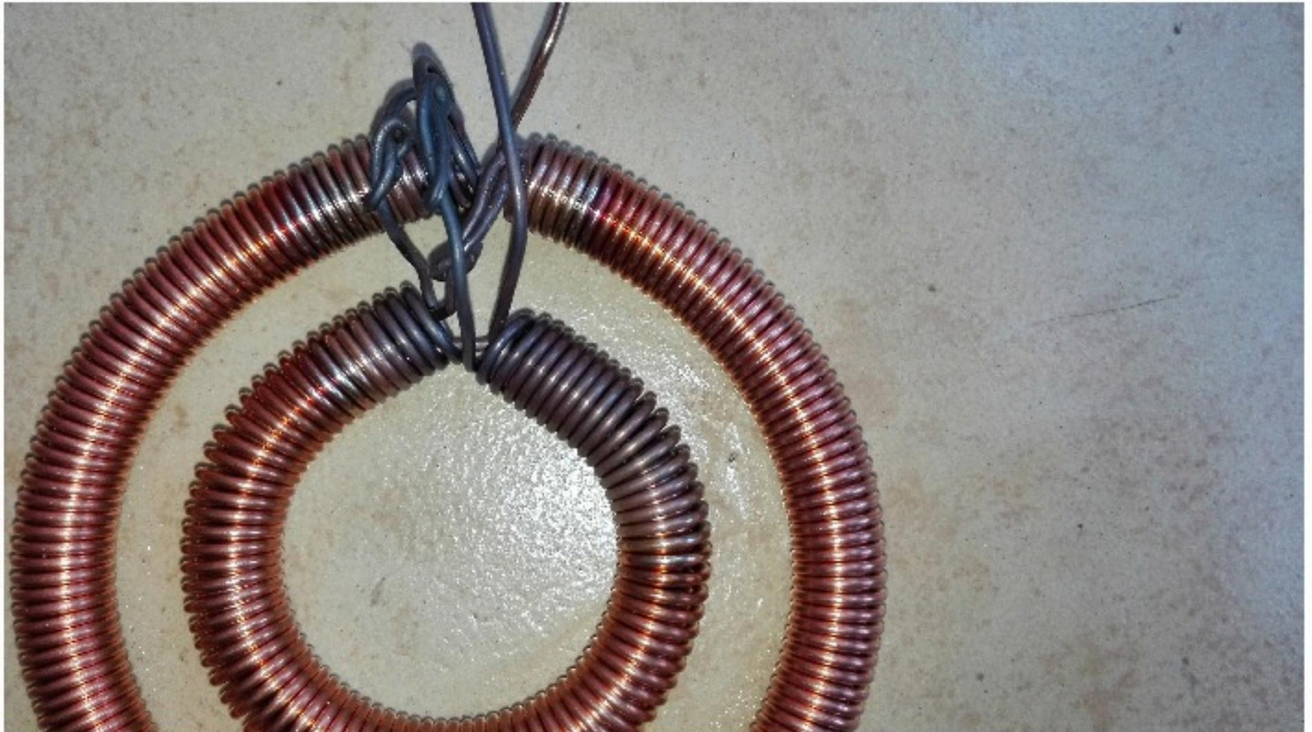
Move the flame up after completing the center loop and start moving counter clockwise around the outer loop.
