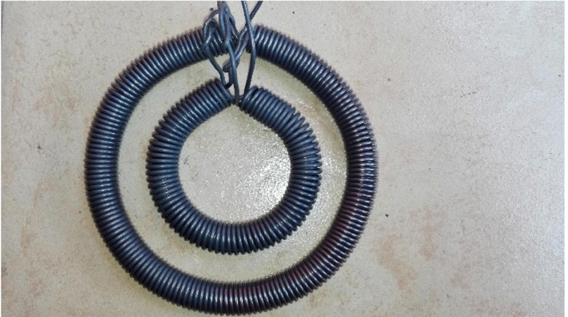
Do a similar process on the other side while still warm but of opposite direction on every loop to have a consistent flow of heat and nano material movement. An optional double flame opposite each other moving together while the coil is hanging on wire on its two terminals can do a single pass process both sides together, saving production time.
