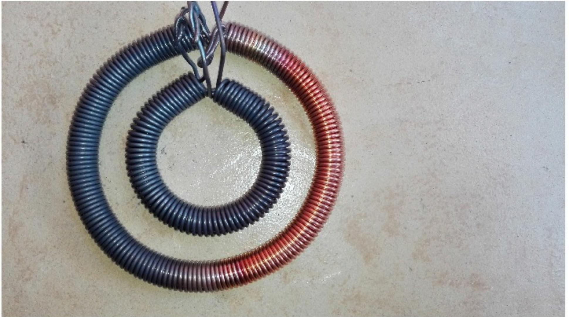
Ideal surface material is ceramic tile while doing this process. Never use metal surface, it will act as heatsink, resulting to inconsistent coating.
