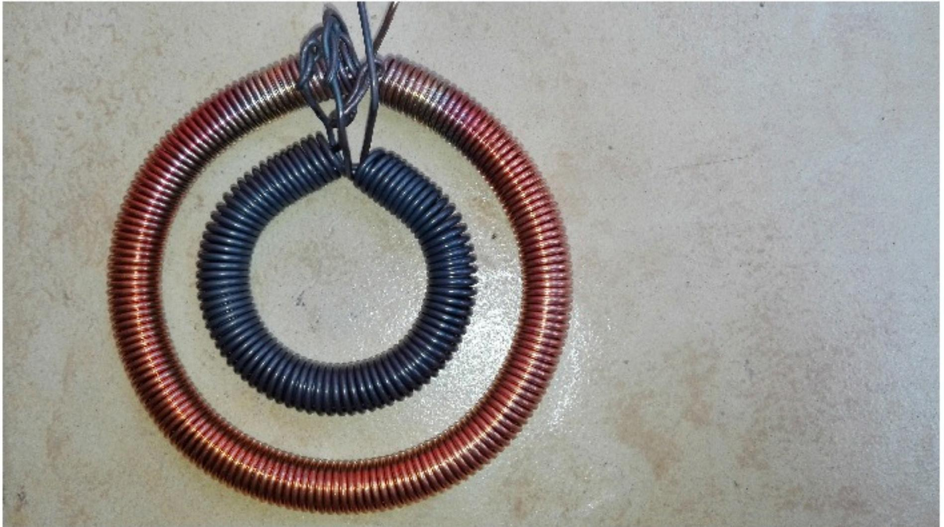
You'll get consistent bluish black color coating when you maintain a consistent temperature by movement speed. The tip of blue part of the flame should be touching the copper like a paint brush.
